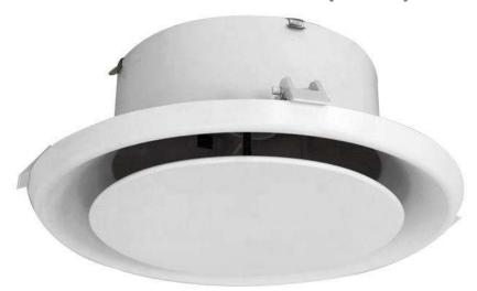
**Description** The LinkedAir Round Diffusers are designed for supply air or exhaust air application. They are manufactured from ABS polymers for everlasting durability. It equips adjustable centre cone which allow for easy airflow or pattern adjustment. It comes with snap down fixing clips for easy installation.
